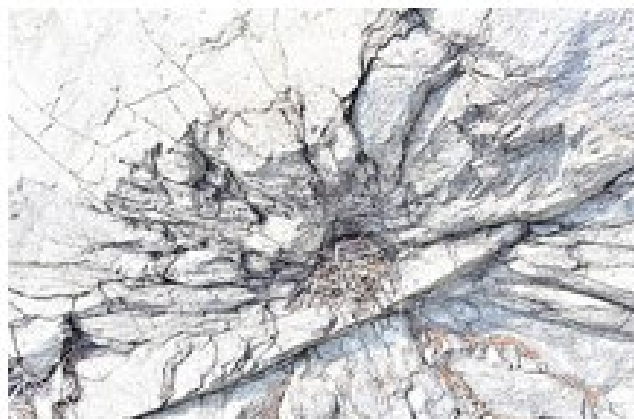
Fig. 2. a: Structure of explosion fracture; b: blast-induced explosion fracture in Lantau, Hong Kong
